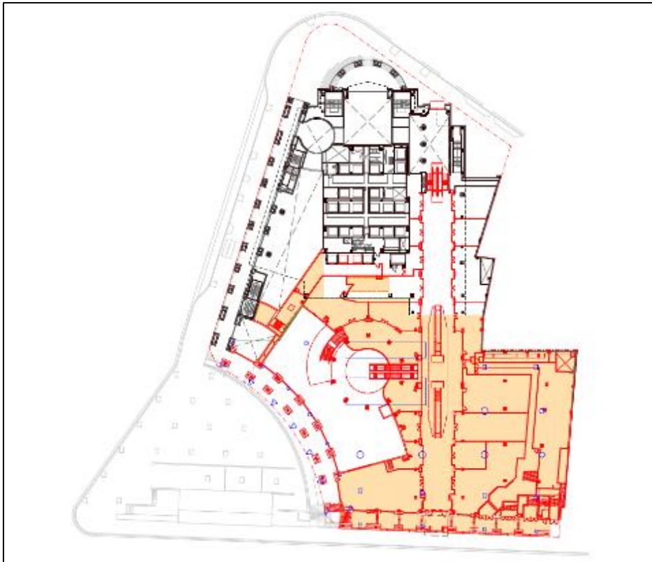
Figure 21: Proposed upper ground floor demolition plan
