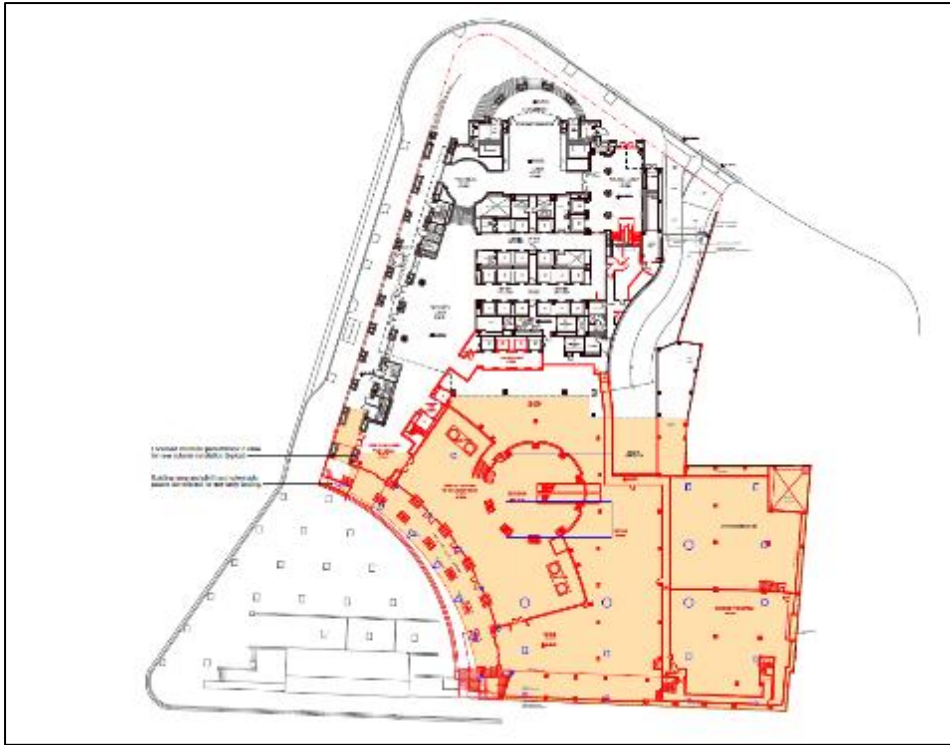
Figure 20: Proposed lower ground floor demolition plan
